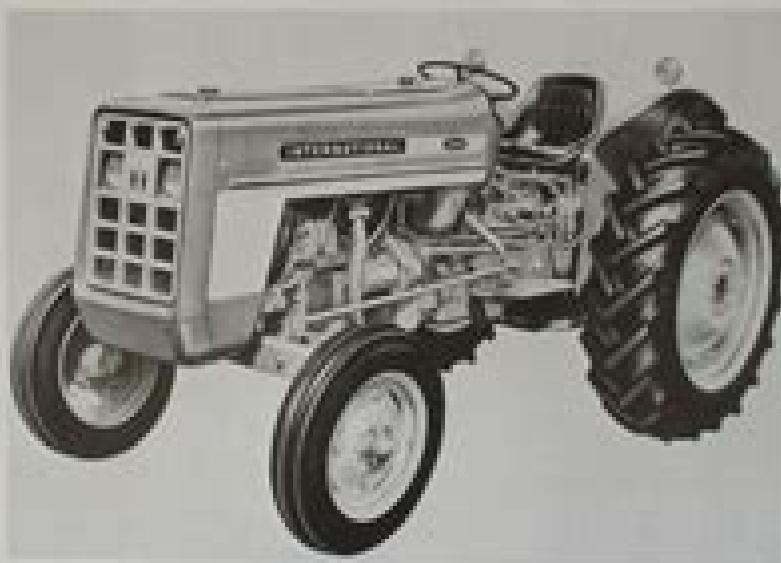
The International 354 tractor is a heavy, low-cost PTO tractor with a choice of gas or diesel engines.
